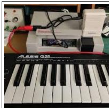
This Nintendo NES console has been modified into a MIDI instrument for writing new music.
