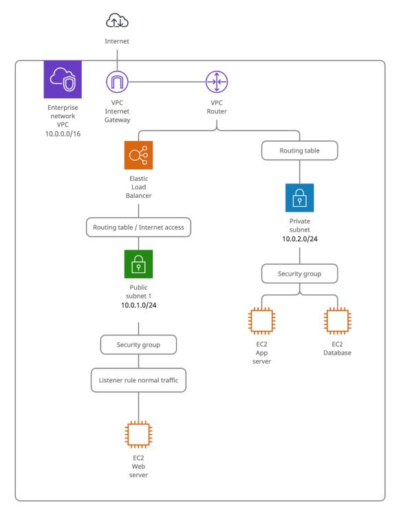
Figure 5 Enterprise Network architecture schematic in Normal Mode
