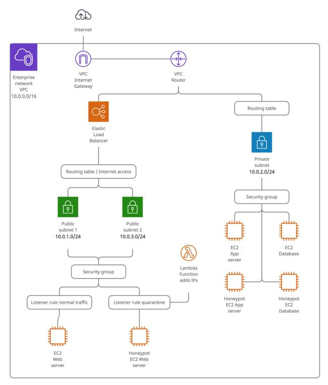
Figure 6 Enterprise Network architecture schematic in Defence mode
